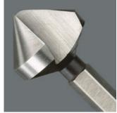
1-flute countersink bits, 90° • Application: Deburring, chamfering and countersinking • ¼" drive suitable for holders as per DIN 3126-D 6.3 (ISO 1173) • Hexagon shaft for very high torque transfer • 1 tip • Guaranteed vibration-free and scratch-free operation • Optimal countersink surface quality • Long service life • Perfect chip removal • High corrosion protection
